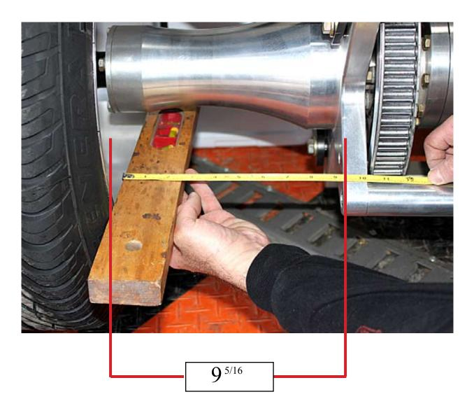
Using straight edge against tire measure distance to outer edge of starplate.
